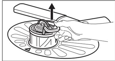
2. Remove the filter (C) out of filter (B).
