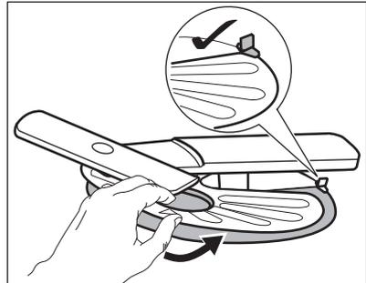
7. Reassemble the filters (B) and (C).
